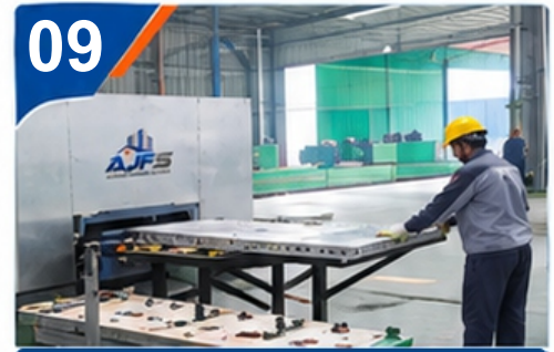
Levelling & Adjustment of Panels
